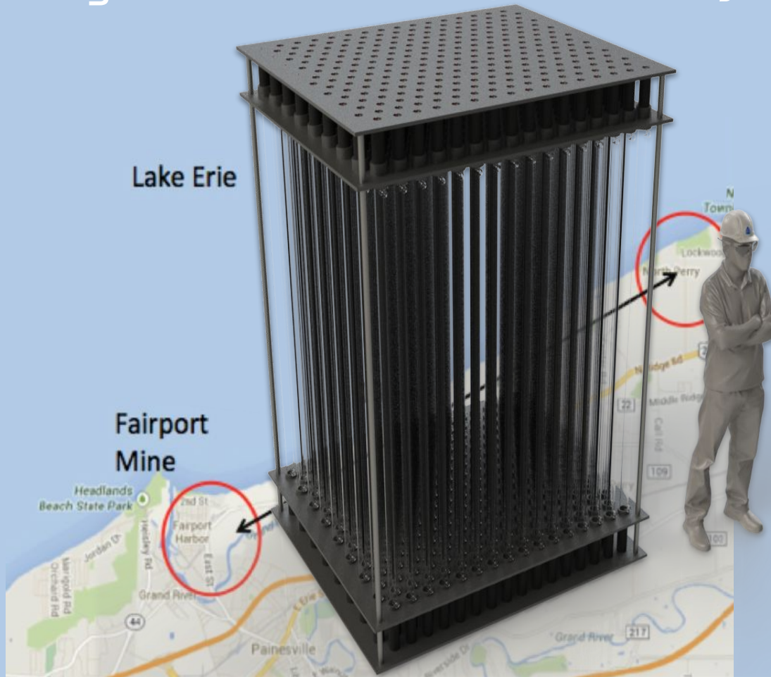
Figure: To scale SolidWorks CAD overlaid with map showing 13km between Morton mine and Perry NPS. An illustrative deployment scenario; was proposed by WATCHMAN: A WAter CHerenkov Monitor for ANtineutrinos
